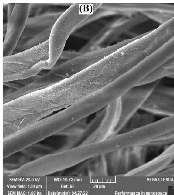
Figure 8: SEM images of (A) an untreated NWCF sample and (B) KC/PEG/K<sup>+</sup>/QNWCF dressing.
