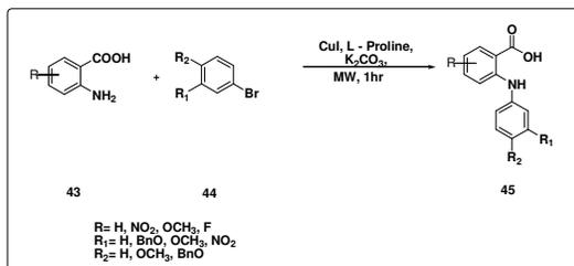
**Figure 11:** Synthesis of *N*-AAs through Microwave-assisted Ullmann reaction
