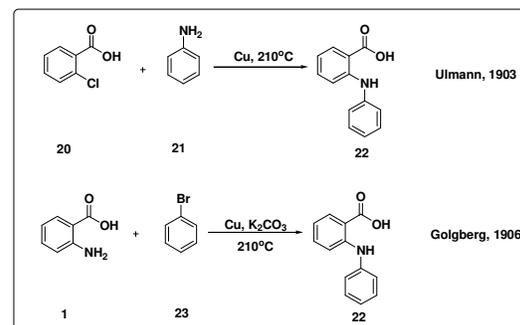
Figure 5: Ullmann-Goldberg coupling reaction for the preparation of N-phenyl AA
