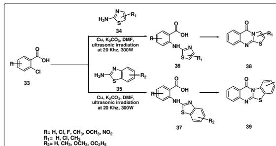
Figure 9: Ultrasonic irradiation synthesis of thiazoloquinazoline and benzothiazoloquinazoline derivatives reported by Docampo *et al*.
