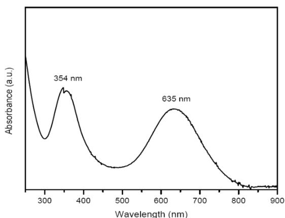
Fig. 5. UV-Vis. absorption spectrum of red-emissive CDs in UPW.
