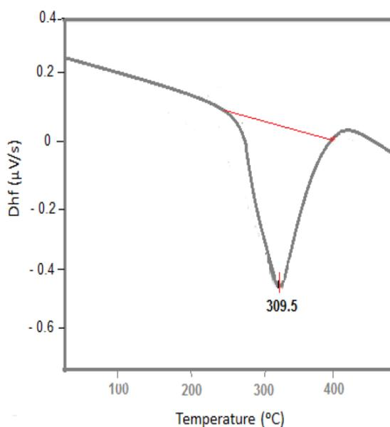
Fig. 3. DSC thermograph of the prepared poly(aspartic acid).
