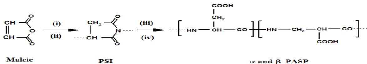
Scheme 1. Synthesis of poly(aspartic acid). (i) DMF, NH<sub>3</sub> gas, 95 °C/ 15 min; (ii) thermal treatment; (iii) NaOH/ 40 °C, 1h; (iv) AcOH pH=3.
