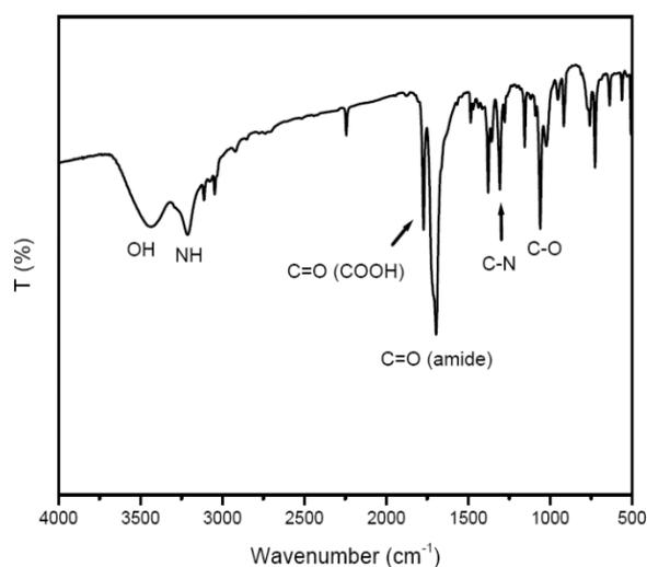
Fig. 1. FTIR spectra of the prepared poly(aspartic acid).
