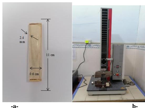
Fig 1: a-shows the tensile strength test sample.b-Shows mechanical properties measuring device (Tensile).
