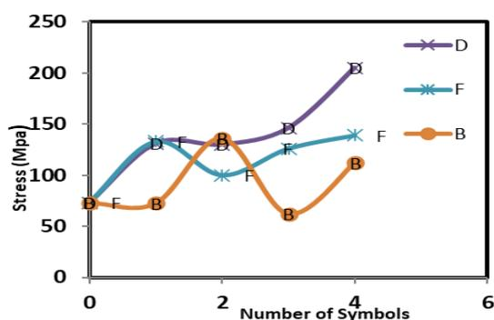
Fig.3. Stress of DOP, polyester, Shilajit and ws.PMMA(groups of D, F, and B).
