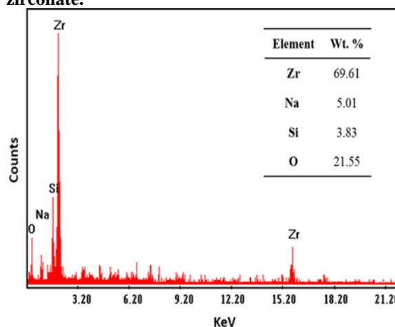
Fig. 4 EDX analysis of sodium zirconate.
