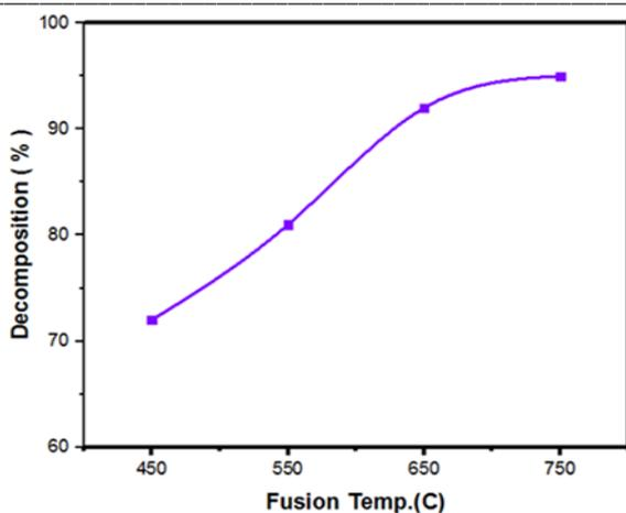
**Fig. 5** Decomposition efficiency versus alkali fusion temperature.
