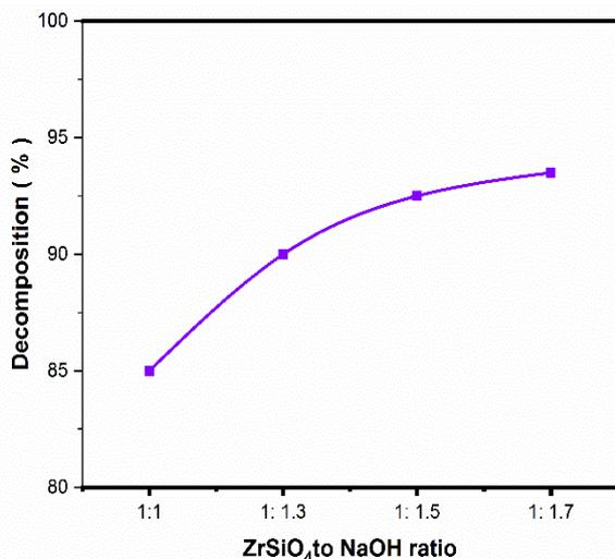
**Fig. 6** Decomposition efficiency versus  $NaOH/ZrSiO_4$  ratio
