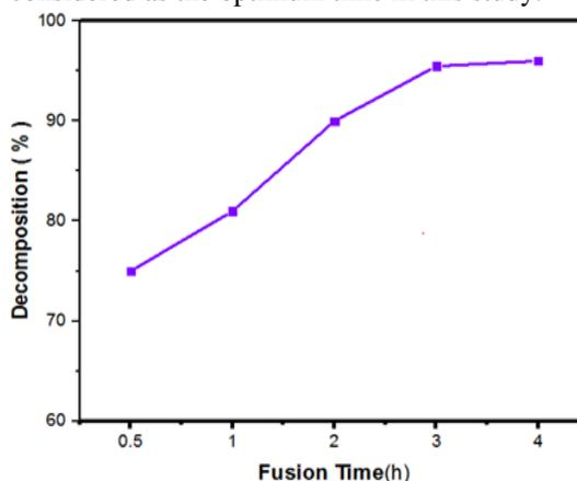
**Fig. 7** Decomposition of zircon versus fusion time
