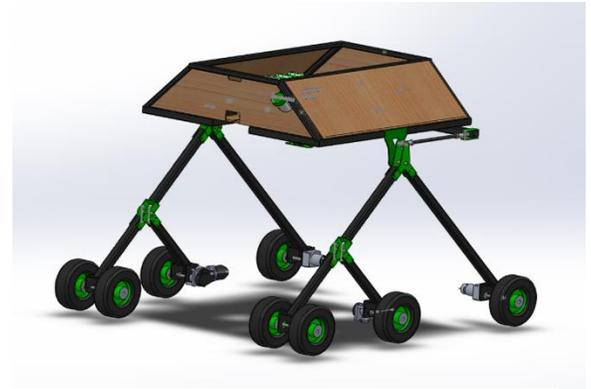
Figure 2: Rocker-Bogie Mechanism
