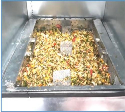
horizontal sample tray was traversed vertically by hot air. (Fig.1b).The dryer system was activated for 30 minutes prior to each experiment in order to obtain the desired steady-state conditions. Using an anemometer (UNIT UT363, China), the air velocity was adjusted to values of (0.1, 1.5, and 2) m/s with an accuracy of 0.1 m/s.
