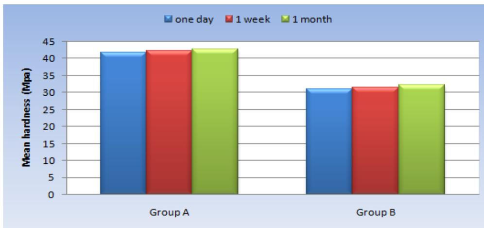
Figure 2: Bar chart representing mean hardness of GI cement and filling without CHX at different time periods.
