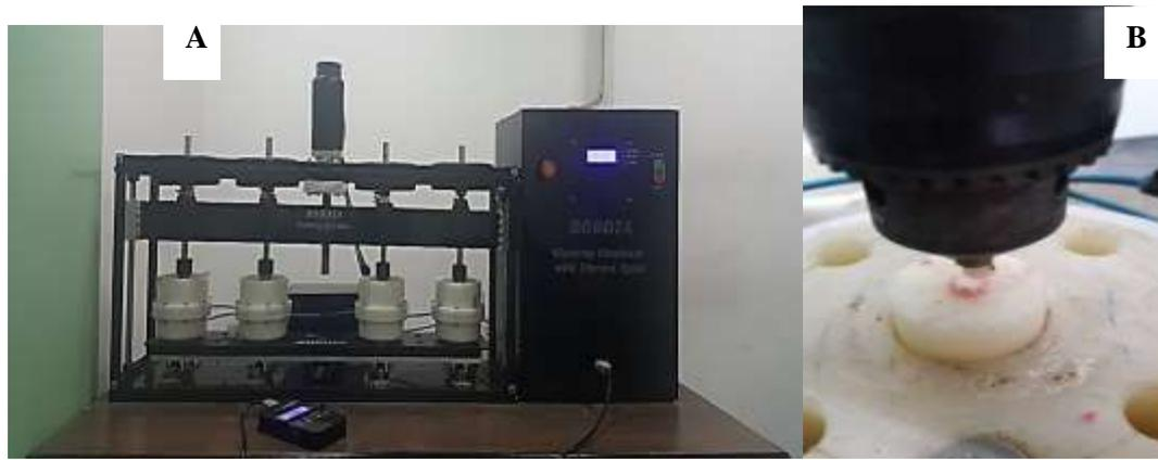
Figure 2: Chewing simulator device (A), disc sample ready for mechanical aging (B).
