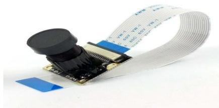
**Figure .5.** Raspberry Pi CAM [6].
