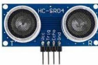
**Figure .8.** Ultrasonic Sensor [10]
