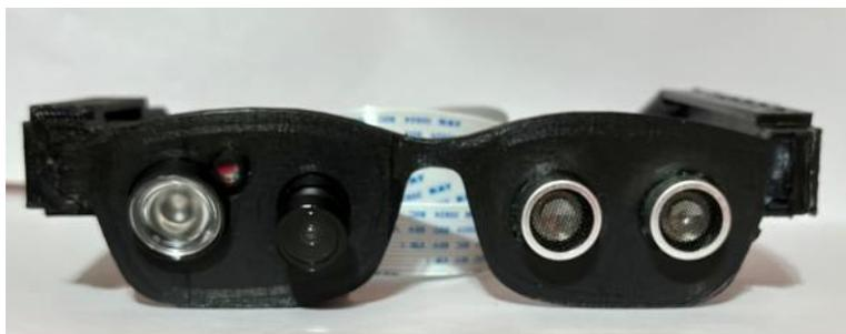
**Figure 9.** AI Amal Glasses prototype.
