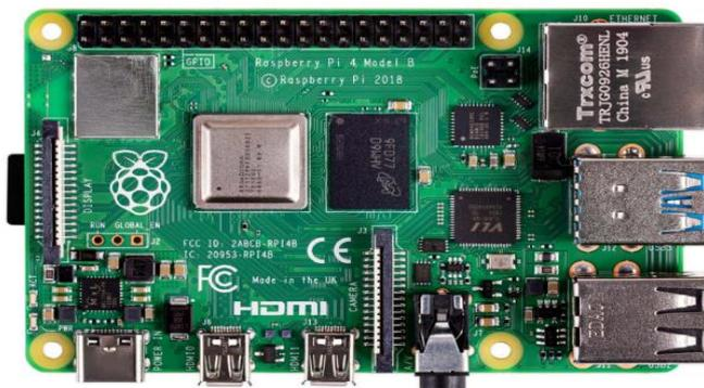
Figure 4. Raspberry Pi 4 Model B and its peripherals connections [6].
