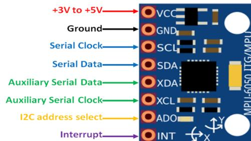
Figure .7. Accelerometer sensor [8].
