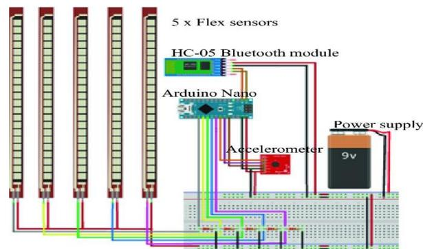
Figure .5. SSG Circuit diagram.
