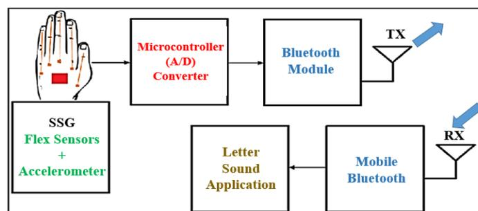
Figure 3. SSG Block Diagram
