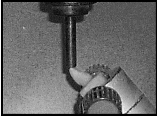
**Figure (5):** Fracture resistance testing using universal testing machine.
