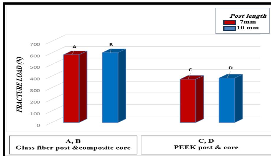
**Figure (6):** Column chart showing the mean values of fracture resistance for both material groups.
