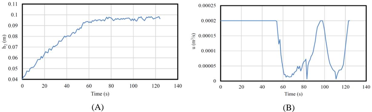
**Figure 12.** Performance of dynamic-SMC with low-pass filter: (A) 0.1 m step response, (B) control signal
