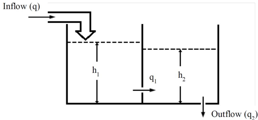
**Figure 1.** Horizontal connected tanks system
