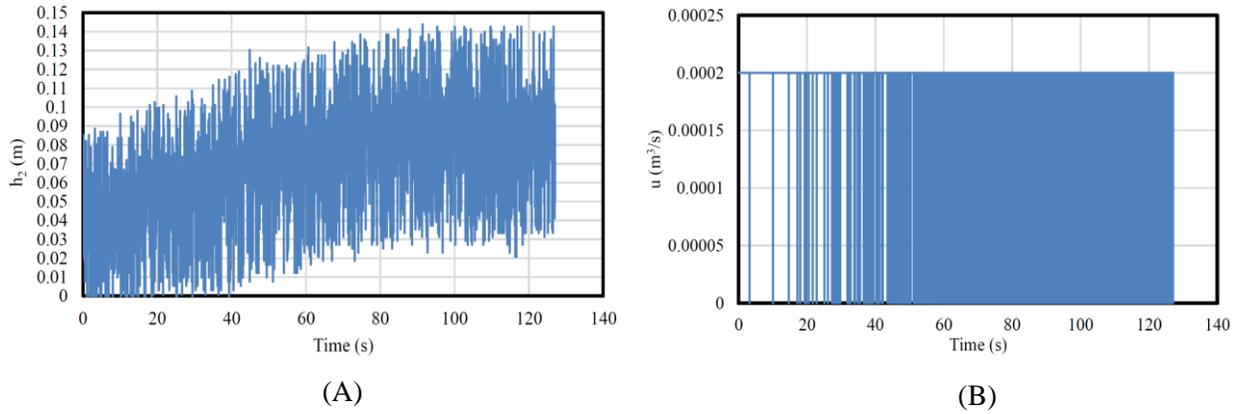
**Figure 9.** Response of PD-SMC when sensor noise is present: (A) Step response, (B) control
