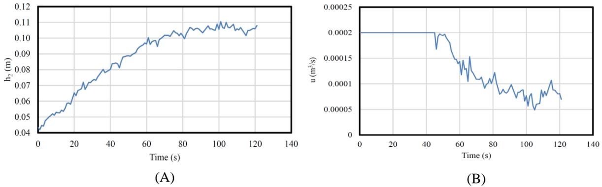
**Figure 11.** Response of PID-SMC with low-pass filter: (A) Step response, (B) control signal
