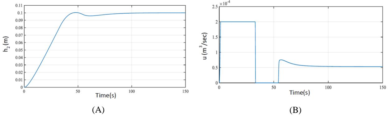
**Figure 5.** Performance of dynamic-SMC (A) 0.1 m step response, (B) Control signal
