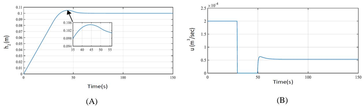
**Figure 4.** Performance of PID-SMC (A) 0.1 m step response, (B) Control signal
