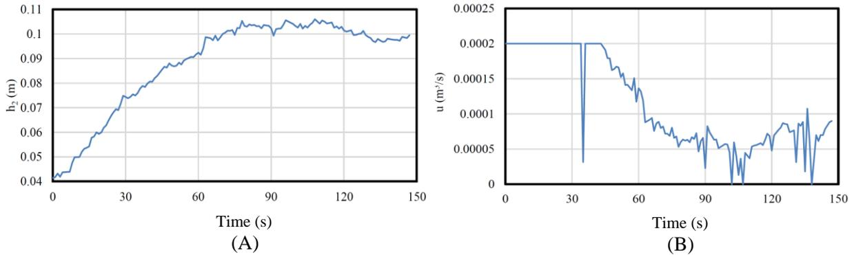
**Figure 10.** Response of PD-SMC with low-pass filter: (A) 0.1 m step response, (B) Control signal
