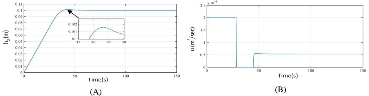
**Figure 3.** Performance of PD-SMC (A) 0.1 m step response, (B) Control signal
