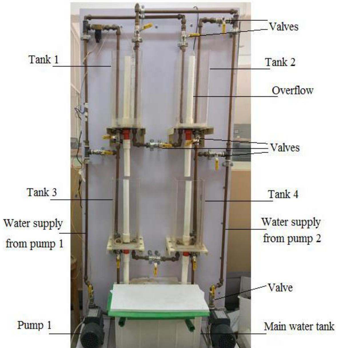
**Figure 6.** Coupled tanks liquid level system
