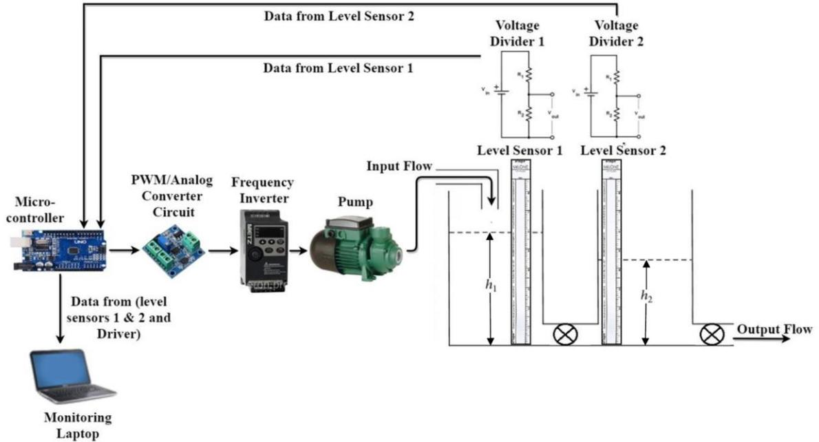
**Figure 7.** Main components of the horizontal coupled tank system
