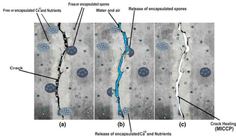
**Figure 4.** Schematic of MICCP crack healing - cracks form in bio-cement with spores and Ca<sup>2+</sup>. Water and air seepage release encapsulated spores and Ca<sup>2+</sup> [6]
