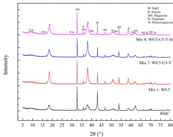
**Figure 3.** XRD patterns of RMC powder, control RMC paste (mix 1), nutritious RMC paste (mix 7), and bio-RMC paste (mix 8) at 28 days, [19].
