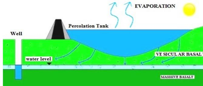
Figure 14: Rainwater Harvesting through Percolation Tank
