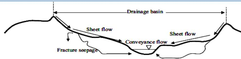
**Figure 3: Sheet and channel flows**
