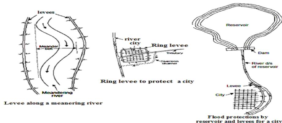
Figure 5: Different procedures for flood mitigation using levees
