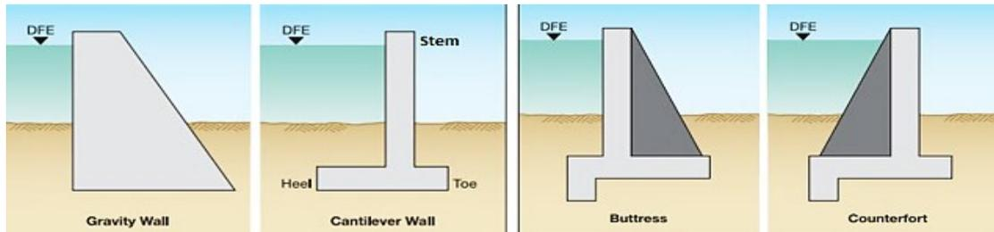
**Figure 8: Types of flood walls**
