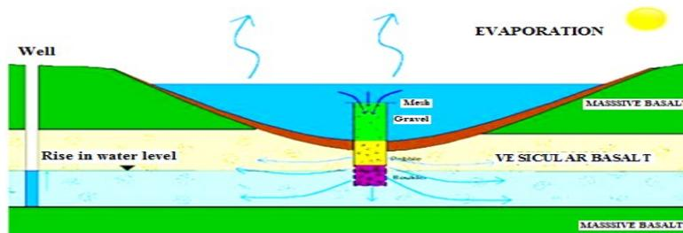
Figure 16: Rainwater Harvesting through Recharge Shaft
