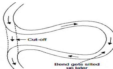
**Figure 10 Cut-off in a meandering river**
