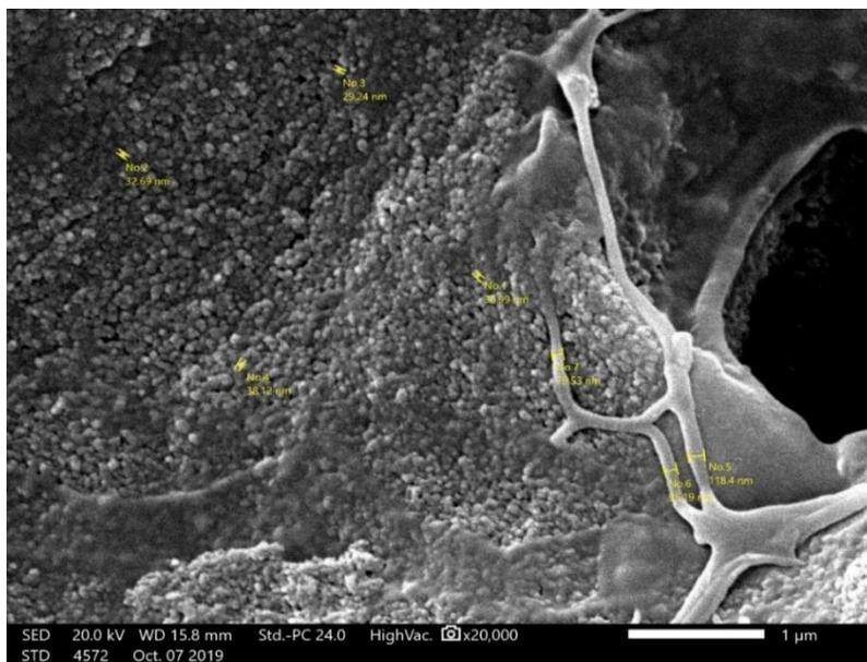
**Plate (1). SEM micrograph of Soft corncob biochar**
