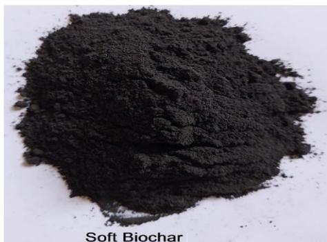
**Figure (1). Picture of the Soft Corn cob biochar used in the present study**
