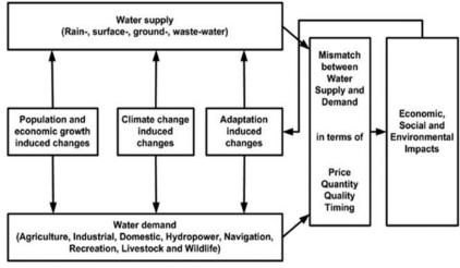
FIGURE 1. The Main Parts of the WEAP
