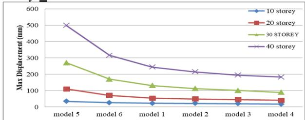
Fig 8: The relation between maximum displacement in the x direction with different models
