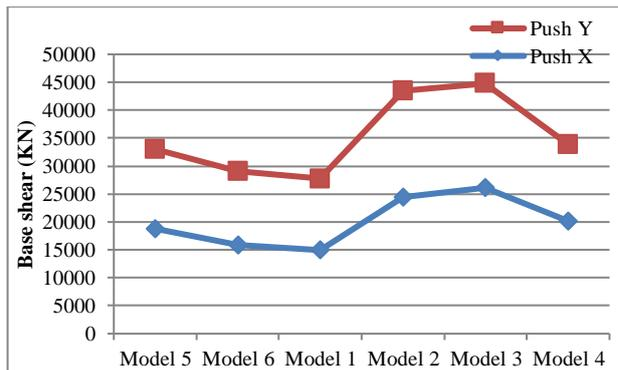
Fig 29: The Base shear for all models in Pushover in both X and Y directions in seismic zone 3.
