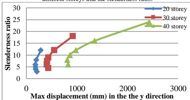
Fig 13: The relation between maximum displacement in the y direction in different storeys and the slenderness ratio
