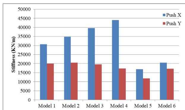
Fig 25: The effective stiffness for all models in Pushover in both X and Y directions.
