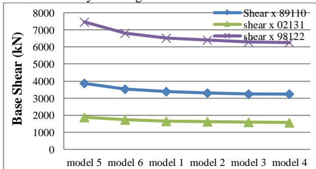
Fig 18: The relation between base shear and different models in various seismic zones (40-storey buildings)
