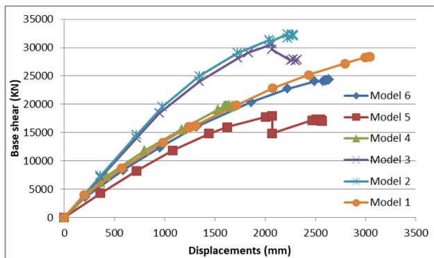
Fig 22: The relation between base shear and maximum displacements in Pushover analysis in Y direction.
