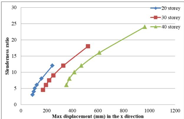
Fig 12: The relation between maximum displacement in the x direction in different storeys and the slenderness ratio.
