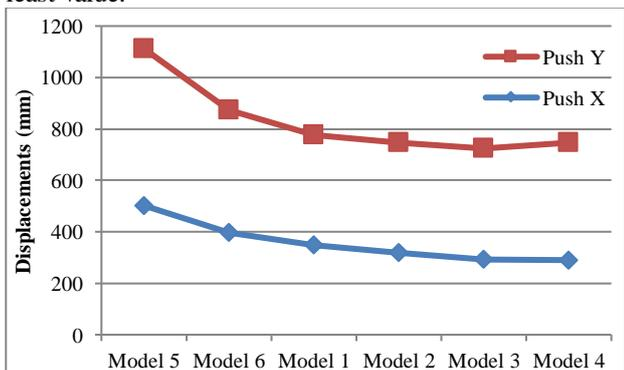
Fig 28: The displacements for all models in Pushover in both X and Y directions in seismic zone 2B
