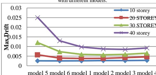
Fig 17: The relation between maximum drift in the y direction with different models
