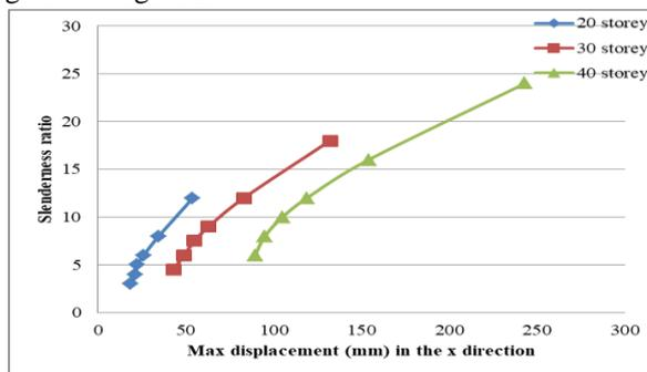
Fig 5: The relation between maximum displacement in the x direction in different storeys and the slenderness ratio
