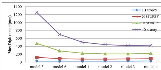
Fig 9: The relation between maximum displacement in the y direction with different models
