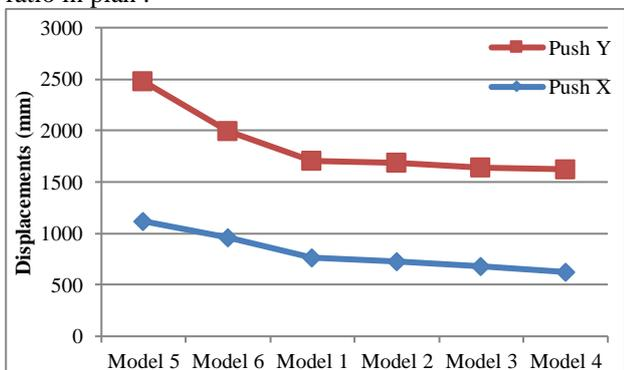
Fig 27: The displacements for all models in Pushover in both X and Y directions in seismic zone 3
