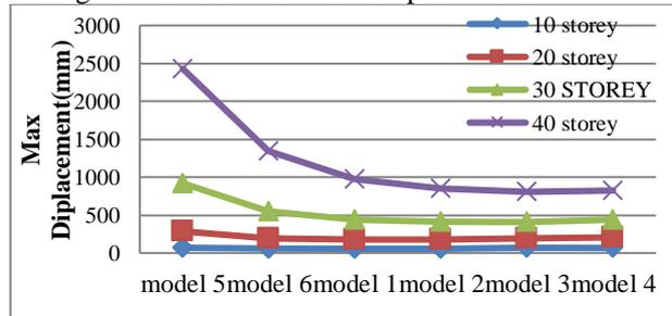
Fig 16: The relation between maximum displacement in the y direction with different models.
