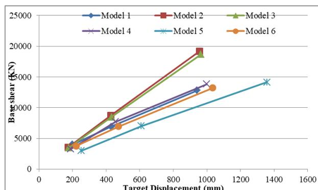
Fig 24: The relation between base shear and Target displacements in Pushover analysis in Y direction in various seismic Zones.
