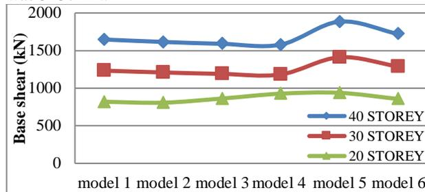
Fig 19: The base shear of different models and storeys
