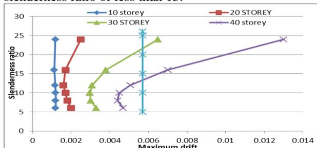
Figure 11: The relation between maximum drift and slenderness ratio for different storeys
