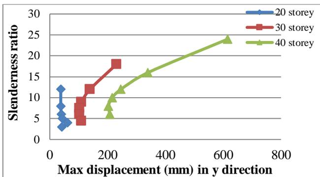
Fig 6: The relation between the maximum displacement in y direction in different storeys and the slenderness ratio
