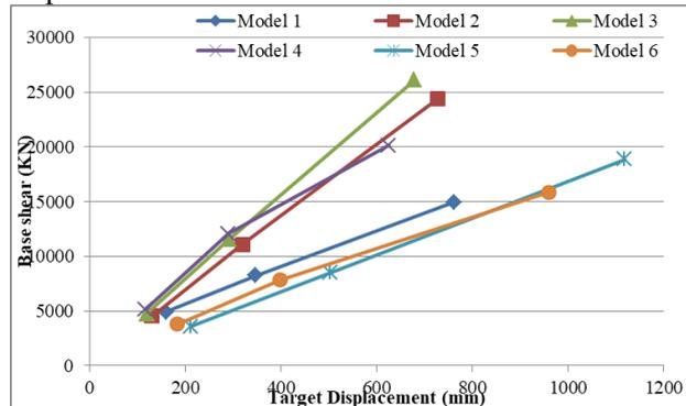
Fig 23: The relation between base shear and Target displacements in Pushover analysis in X direction in various seismic Zones.
