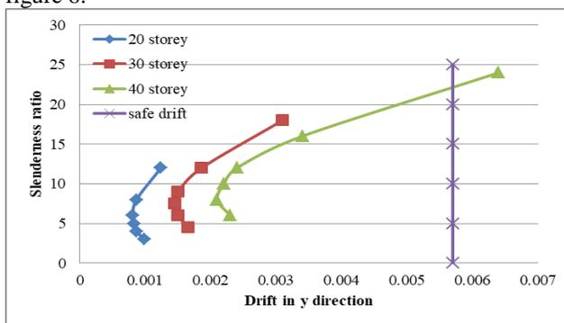
Fig 7: The relation between the maximum drift in the y direction in different storeys and the slenderness ratio
