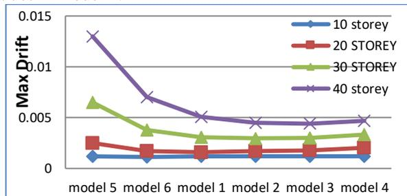
Fig 10: The relation between maximum drift in the y direction with different models
