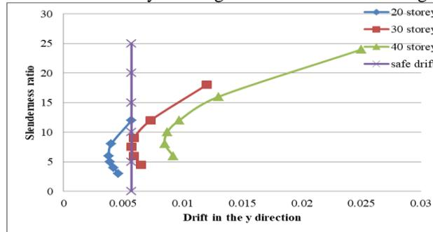
Fig 14: The relation between maximum drift in the y direction with slenderness ratio
