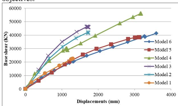
Fig 21: The relation between base shear and maximum displacements in Pushover analysis in X direction.
