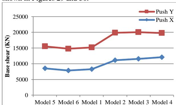
Fig 30.: The Base shear for all models in Pushover in both X and Y directions in seismic zone 2B.
