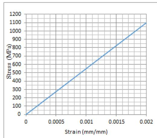
(c) Stress-strain curve for GFRP bars
