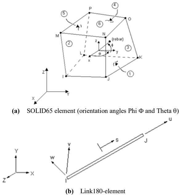
FIGURE 1. Idealization for beams by ANSYS [17]
