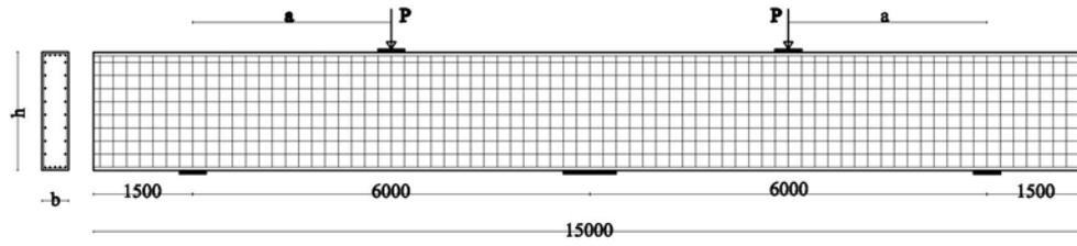
FIGURE 7. Details of the typical beam used for parametric study (mm.)
