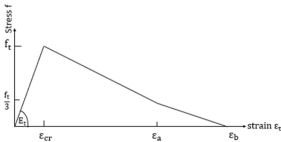
(a) Concrete stress-strain curve in tension
