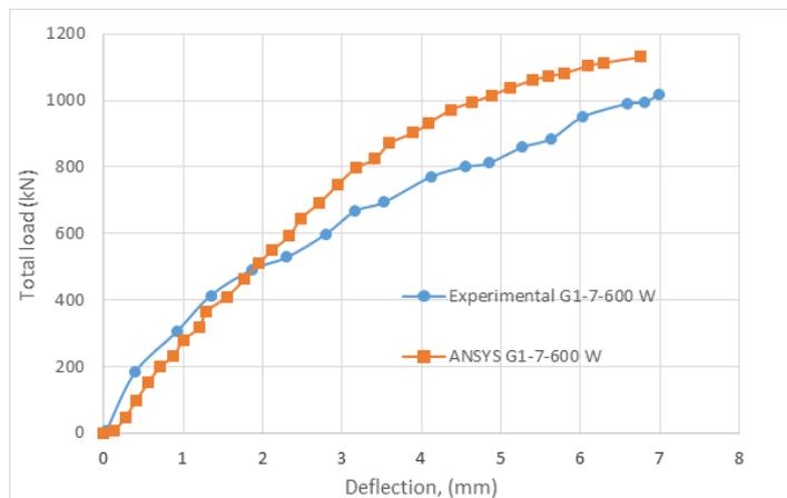
FIGURE 4. Numerical vs. experimental load-deflection curves for beam G1.7-600-W Zinkaah et al. [18]
