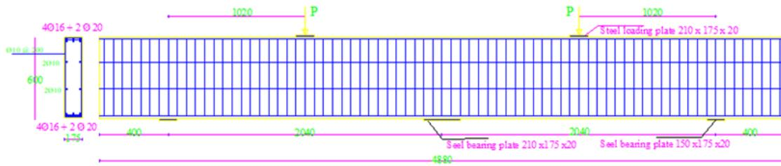
(a) Concrete dimension and cross-section
