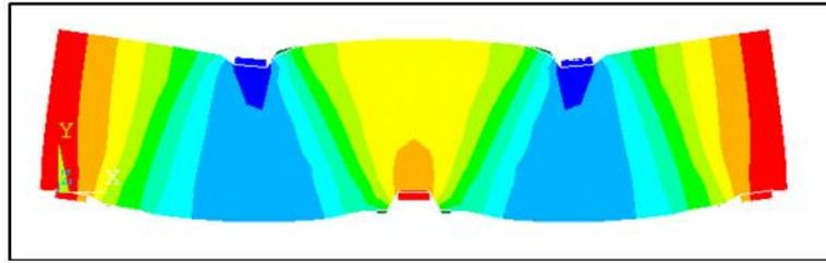
FIGURE 5. Deformed shape of beam G1.7-600-W Zinkaah et al. [18] at 100% failure load
