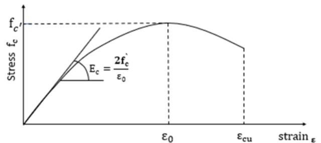
(b) Concrete stress-strain curve in compression
