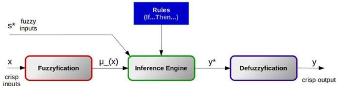
Figure 3: Fuzzy control system diagram [51]
