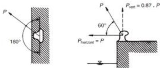
Fig 2 Bollard load direction and value (ICE, 2014)
