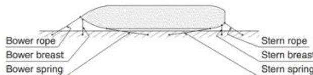
Fig 1 General mooring arrangement for a ship to a berth by way of bollards (ICE, 2014)
