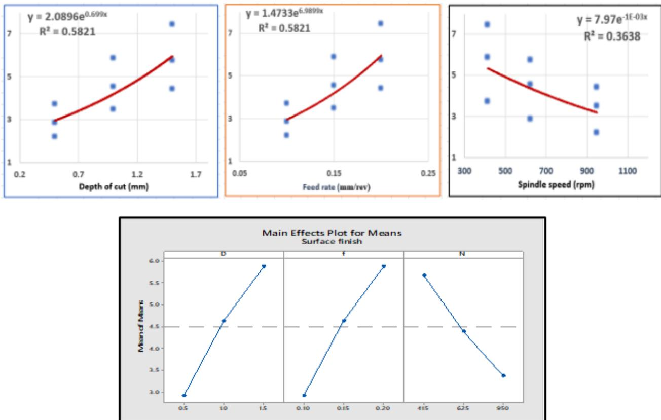
**Fig 7.** ANOVA results for process parameters analysis
