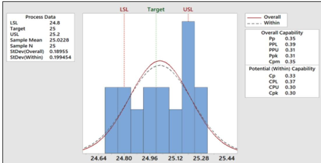
Fig 8. Process capability analysis (before improvement).
