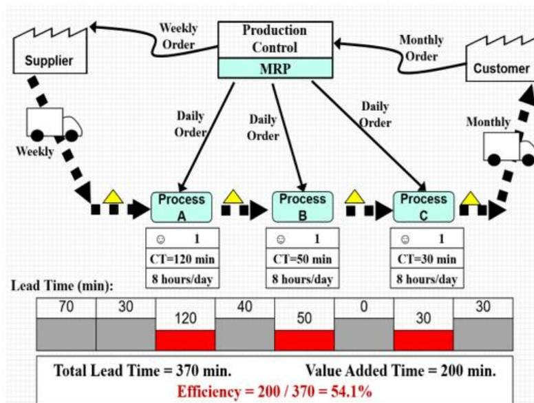
Fig 18. Value stream mapping (After improvement)
