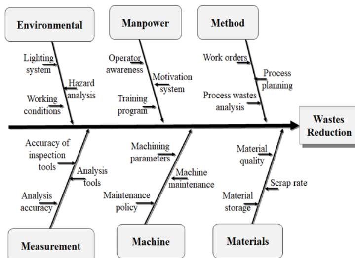
Fig 14. C&E diagram for process wastes reduction.
