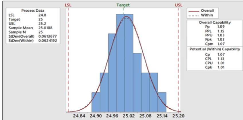
Fig 17. Process capability analysis (After Improvement)
