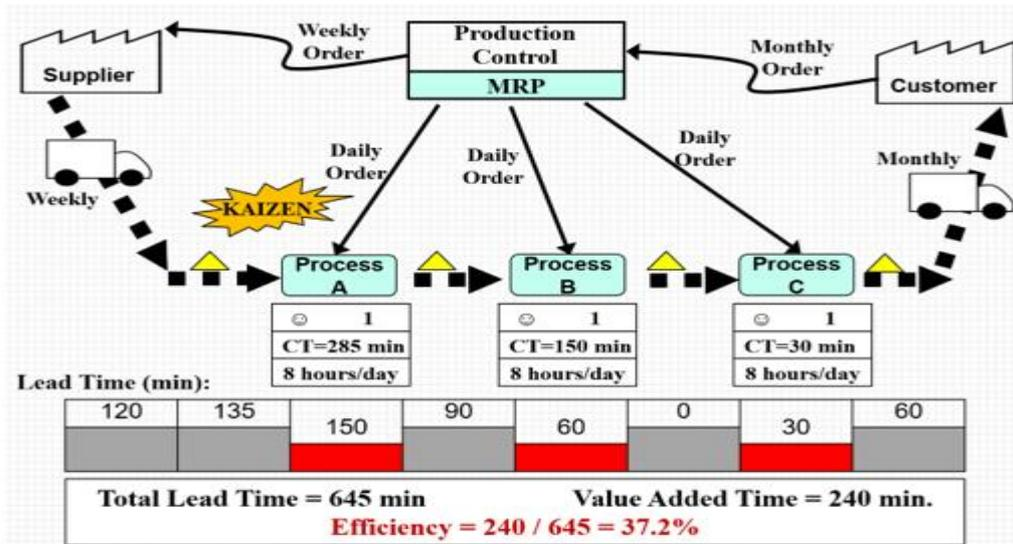
Fig 10. Value stream mapping (before improvement).
