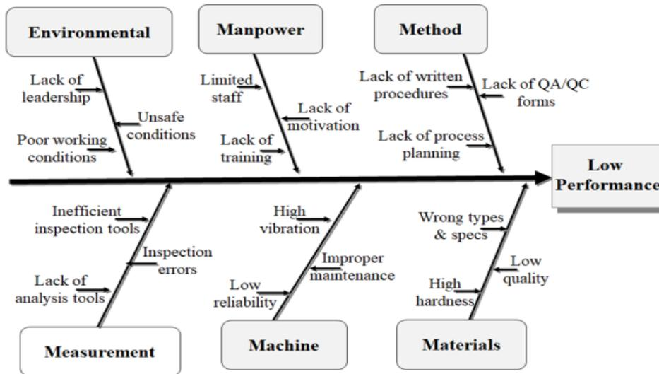
Fig 12. C&E diagram for low process performance.
