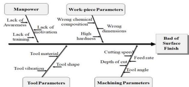
**Fig 6.** C&E diagram for bad of surface finish
