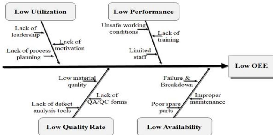
Fig 13. C&E diagram for low overall equipment effectiveness (OEE).
