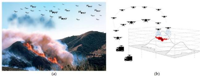
Fig3:(a,b) Representations of the proposed firefighting system based on the use of a swarm of collaborative UAVs.
