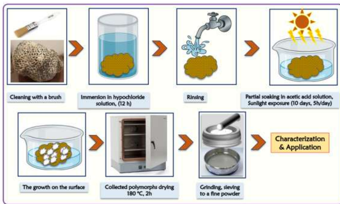
Figure 1. Procedures used for the preparation of the Polymorphs. Starting with the coralline limestone, heading to the meersion, and finally seizing a powder ready for further analysis.
