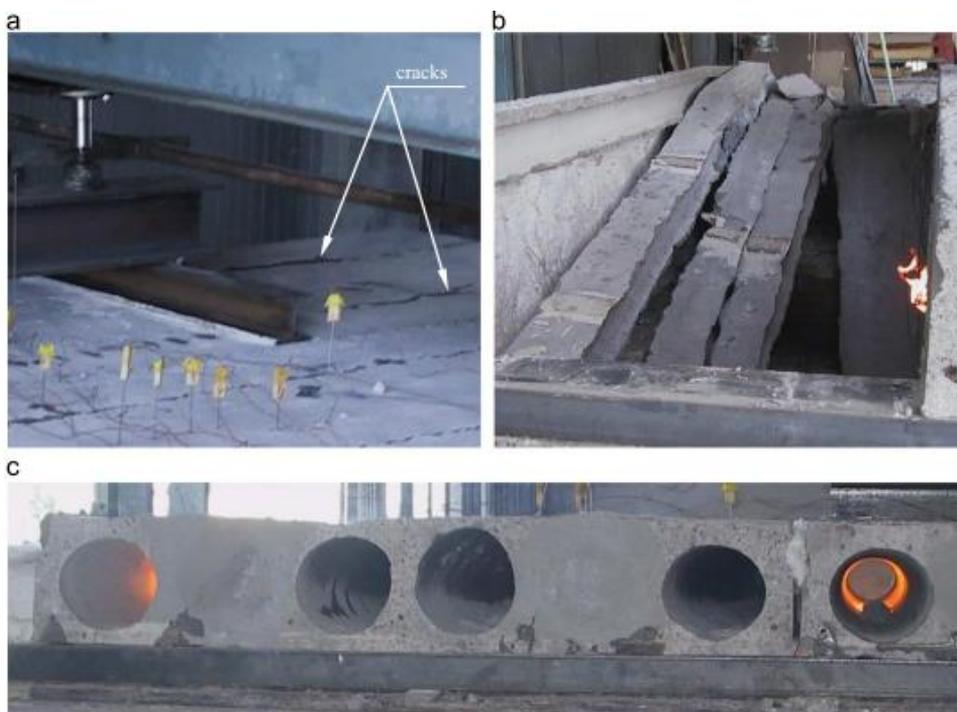
Figure 6: The spalling of concrete is occurred [ 28]
