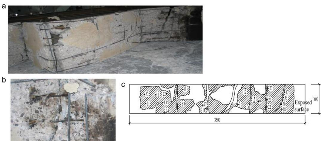
Figure 5. simply-supported slab: (a) spalling of exposed surface (b) reinforcement damage (c) concrete spalling (Spalling is shown by a hatched region, and the number there indicates the depth to which spalling may go) [21].
