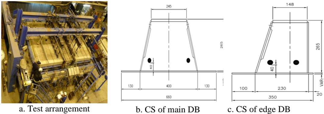
Figure 4: Test arrangement CS of the DB [13]
