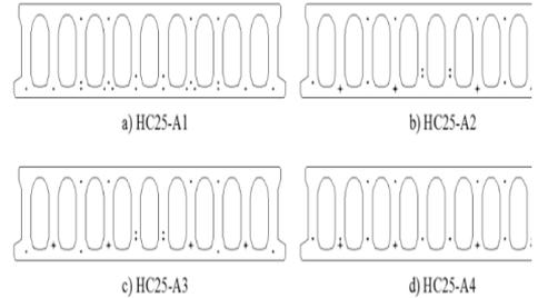
Figure 10: CS and reinforcement arrangement of tested HCS slabs [12]
