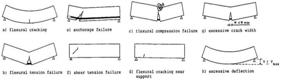
Figure 13: Possible failure mechanisms for HCS [23]
