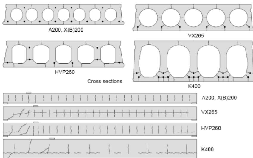
Figure 14 crack patterns for HSC [8]
