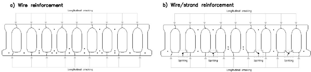
Figure 12: the cracking pattern [12]
