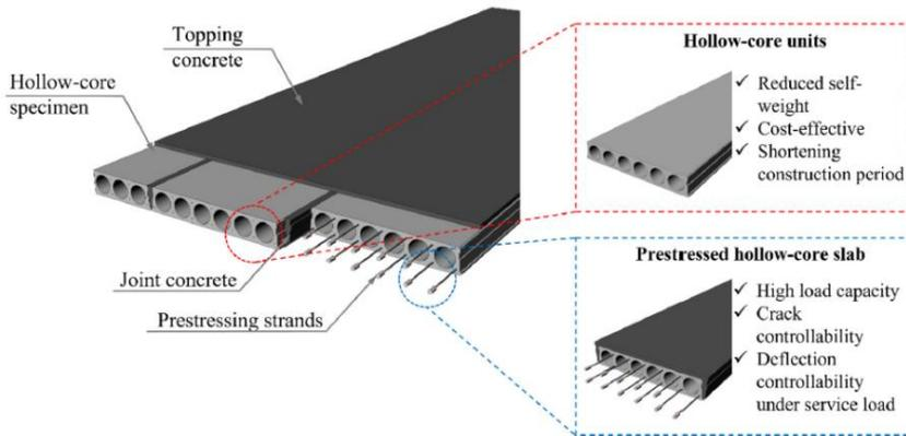
Figure 1. Prestressed hollow-core slabs [1]
