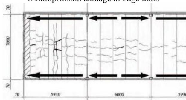
c Slabs restraint creates a compressive strip
