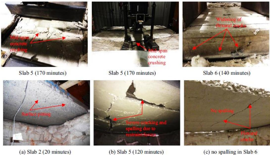
Figure 7. Failure modes and typical spalling in HCS under fire exposure [19]
