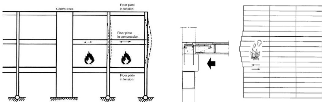
Figure 2.a: Elevation demonstrates blocking impact of the edge construction
