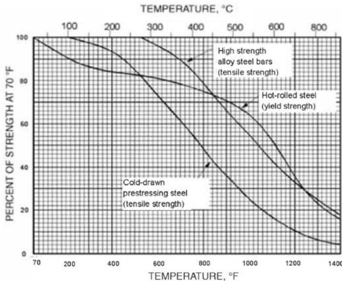
Figure 8: Strength of flexural reinforcement steel bar and strand at high temp. [22]
