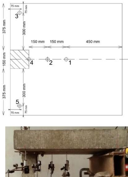
Fig. 8. LVDT locations at lower face.
