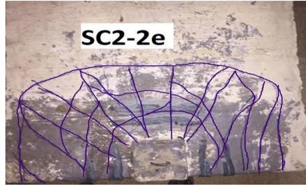
Fig. 36. Pattern of cracking for specimen (SC2-2e).
