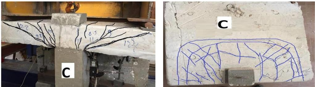
Fig. 30. Cracking pattern for specimen (C).
