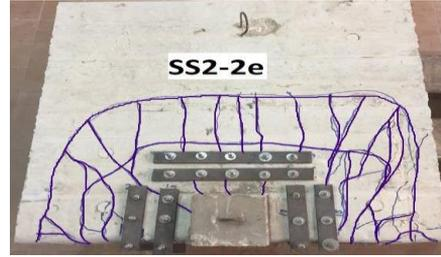
Fig. 44. Pattern of cracking for specimen (SS2-2e).
