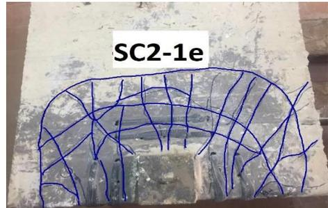
Fig. 35. Pattern of cracking for specimen (SC2-1e).
