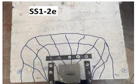
Fig. 43. Pattern of cracking for specimen (SS1-2e).
