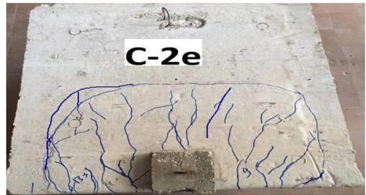
Fig. 32. Pattern of cracking for specimen (C-2e).
