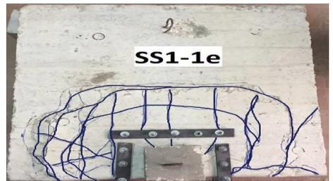
Fig. 41. Pattern of cracking for specimen (SS1-1e).
