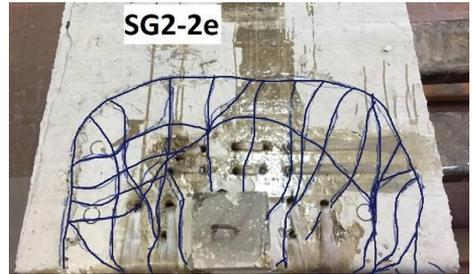
Fig. 40. Pattern of cracking for specimen (SG2-2e).
