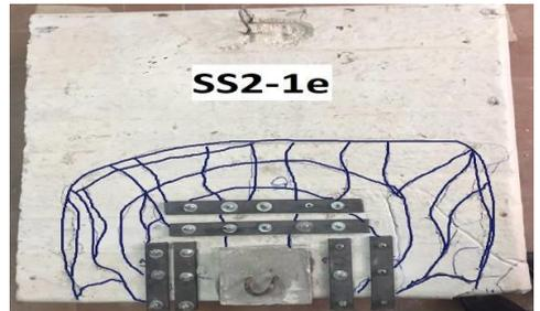
Fig. 42. Pattern of cracking for specimen (SS2-1e).
