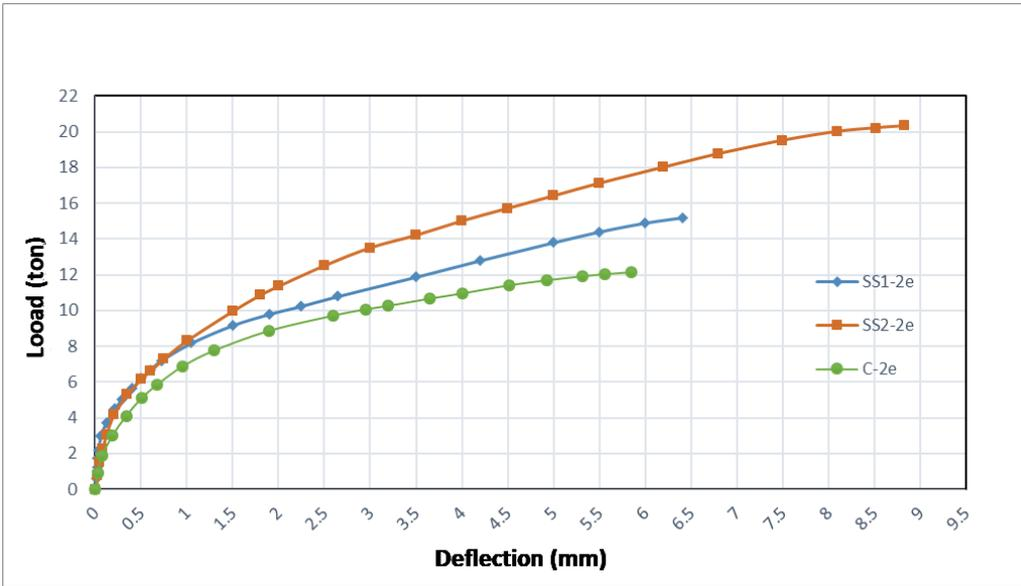
Fig. 19. Effect of rows number of strengthening steel links with eccentricity value (2e).
