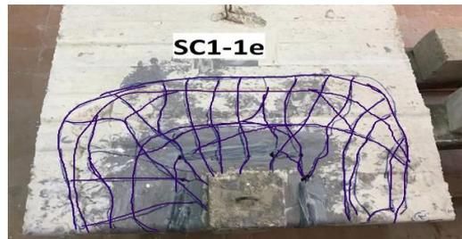
Fig. 33. Pattern of cracking for specimen (SC1-1e).
