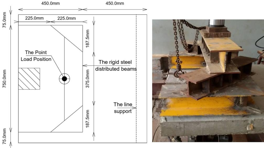
Fig. 7. The used distributed rigid steel beams.
