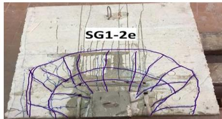
Fig. 38. Pattern of cracking for specimen (SG1-2e).
