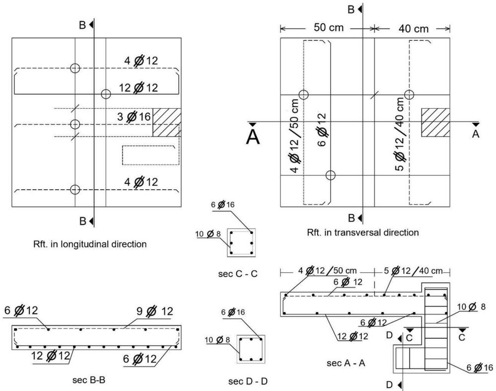
Fig. 2 The specimen's reinforcement.
