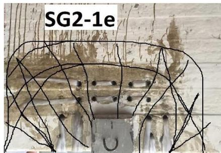
Fig.39. Pattern of cracking for specimen (SG2-1e).
