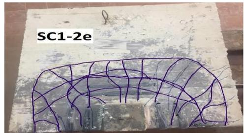
Fig. 34. Pattern of cracking for specimen (SC1-2e).
