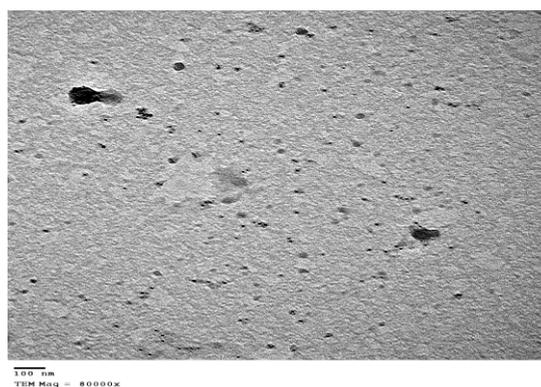
**Fig.2:** TEM image of the prepared Ag NPs particles in the polymermatrix
