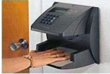
**Fig. 6. Scanner for hand geometry**
