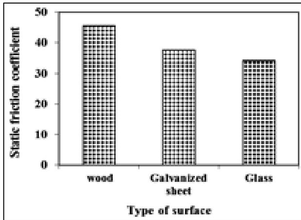
Fig. 7. Static friction coefficient for white Mulberry fruits on different material surface.
