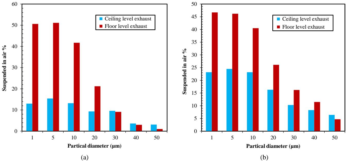
Figure 7: Relation between particle diameters and particles suspended in the air with different exhaled velocities (a) Exhaled velocity 0.12 m/s, (b) Exhaled velocity 2 m/s [54].
