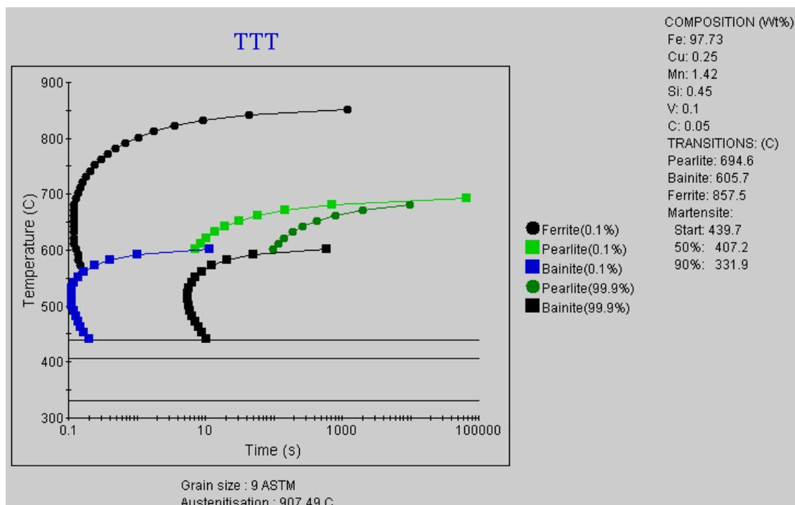
**Fig. 2: Diagram simulated by using JMatPro software: time-temperature transformation diagram (TTT).**
