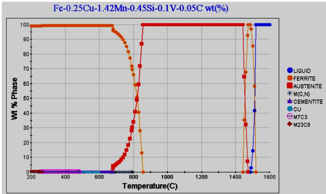
**Fig. 1: Simulated diagram obtained by using JMatPro software: amount of phases as a function of temperature.**
