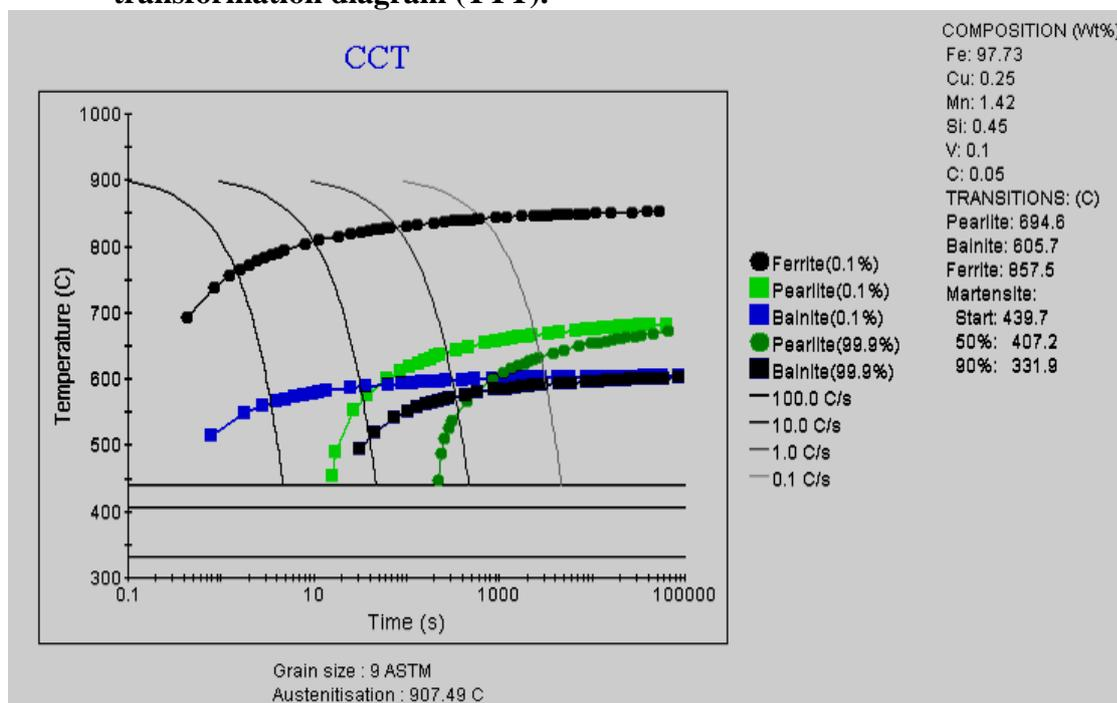
**Fig. 3: Diagrams simulated by using JMatPro software: Transformation diagram in continuous cooling (CCT).**
