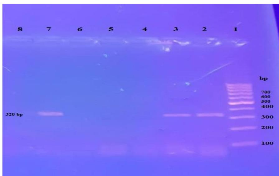
**Fig. 2:** Gel electrophoresis showing the amplified product of the *mcr-1* gene (320 bp). Lane 1: 100 bp DNA ladder (Cleaver Scientific, UK). Lane 2-3: *mcr-1* positive isolate; Lanes 4–6: negative isolates; Lane 7: positive control for *mcr-1* gene; Lane 8: negative control.
