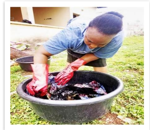
Dipping Fabric into the Prepared Dye.
