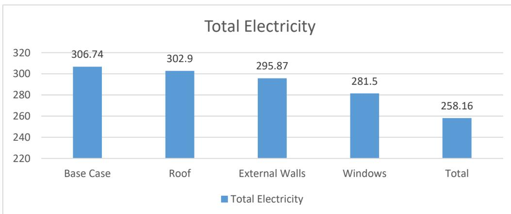
The results of adding VIPs to the external wall insulation and TiO<sub>2</sub> Cladding showed that total energy use was reduced by more than 3.5%. the adding VIPs to the roof reduce about 1.37%.
