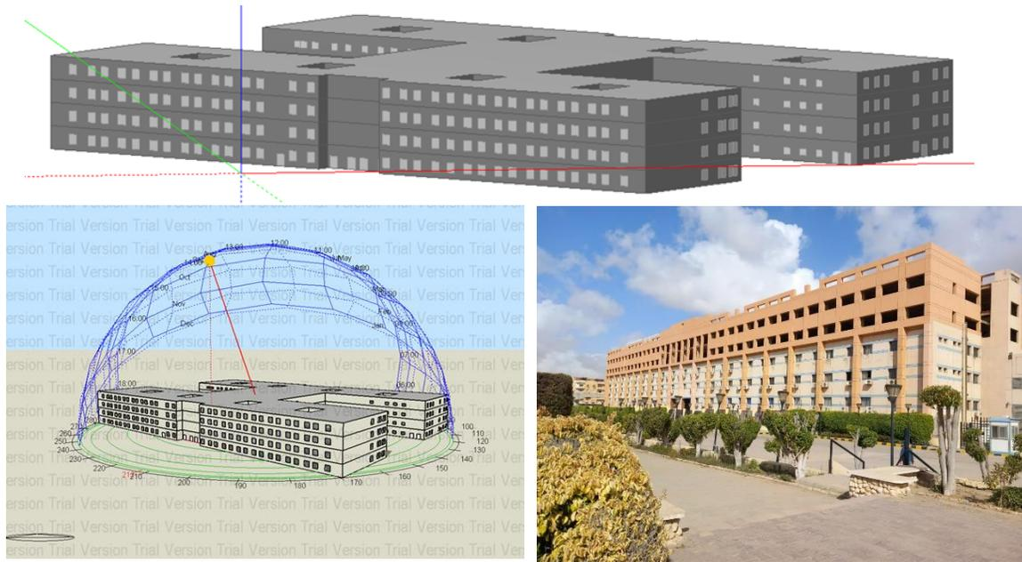
Fig.12 The base case simulation thermal model (3D Model)
