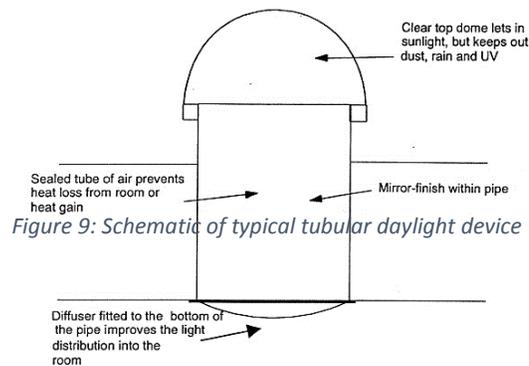
Figure 9: Schematic of typical tubular daylight device
