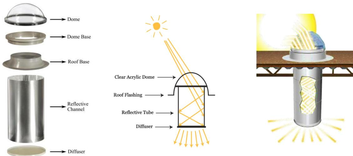
Figure 8: Tubular daylighting device component
