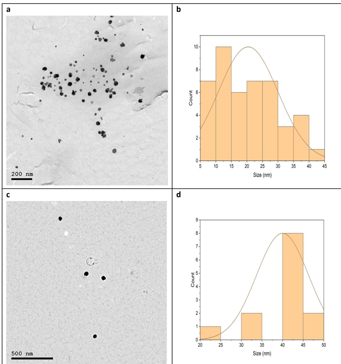
**Fig. 1.** (a) HRTEM image for silver nanoparticles embedded in PVP/ AAm/ Acetic acid/ Glycerol, (b) size distributions of silver nanoparticles for (a) sample, (c) HRTEM image for silver nanoparticles embedded in PVP/ AAm/ Acetic acid, and (d) size distributions of silver nanoparticles for (d) sample.
