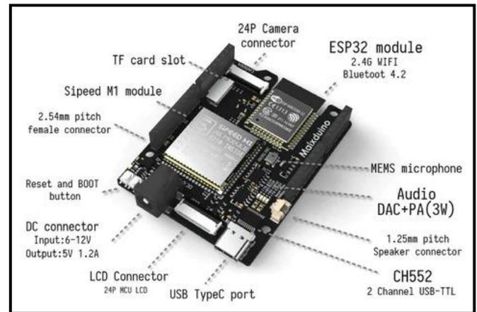
Figure 3: Sipeed Maixduino Kit RISC-V .
