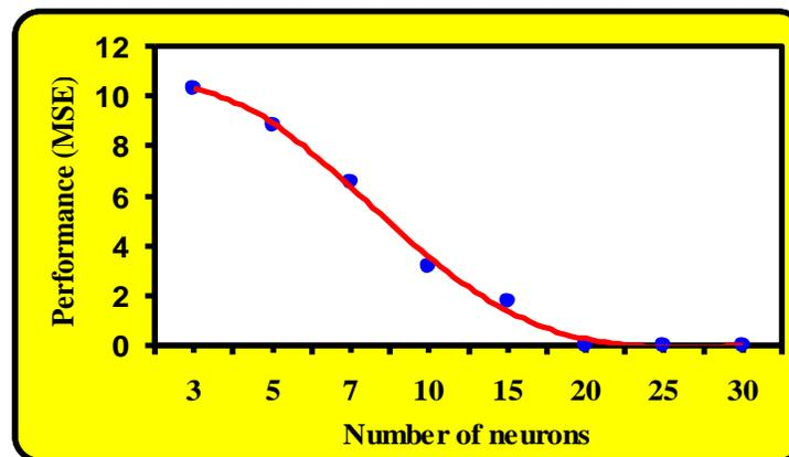
**Figure (1): Relationship between the number of neurons in the hidden layer of the artificial neural network and its performance**
