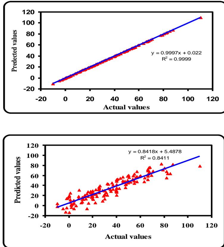
**Figure (3): Actual versus predicted vales using ANN model for twist loss of the weft yarns on Air-Jet weaving machine.**
