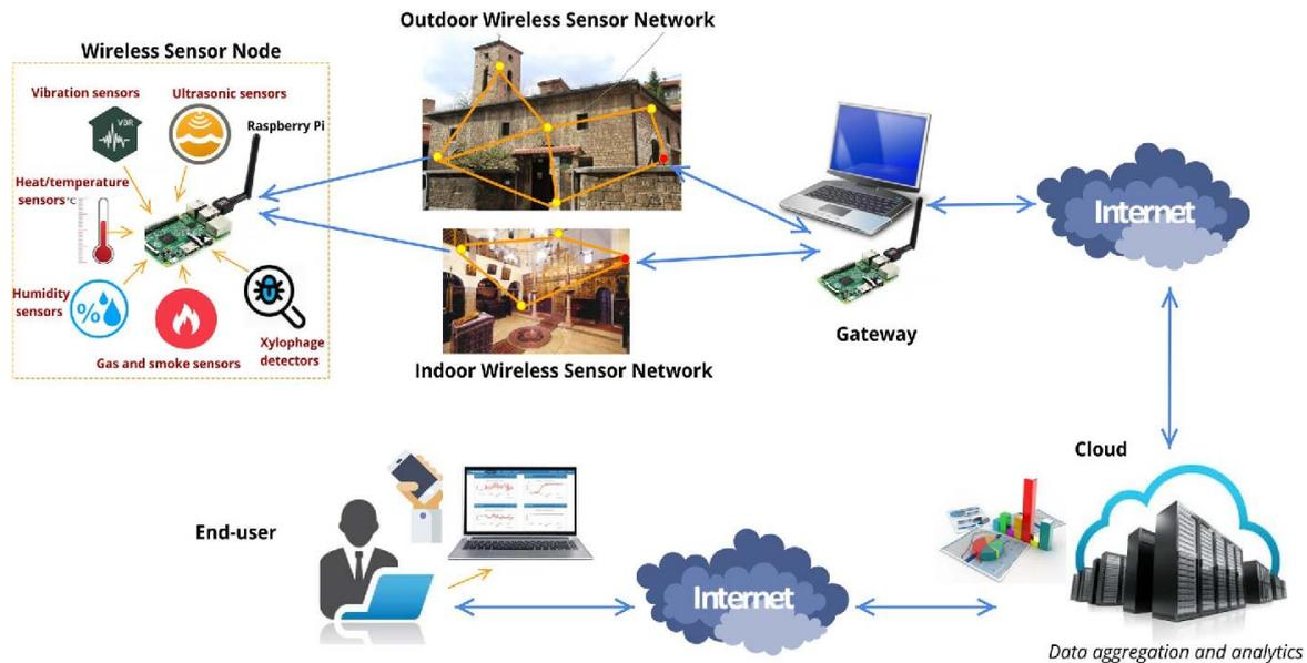
Fig. 12. The general structure of the proposed monitoring system based on (IoT) in the church building[ 32].
