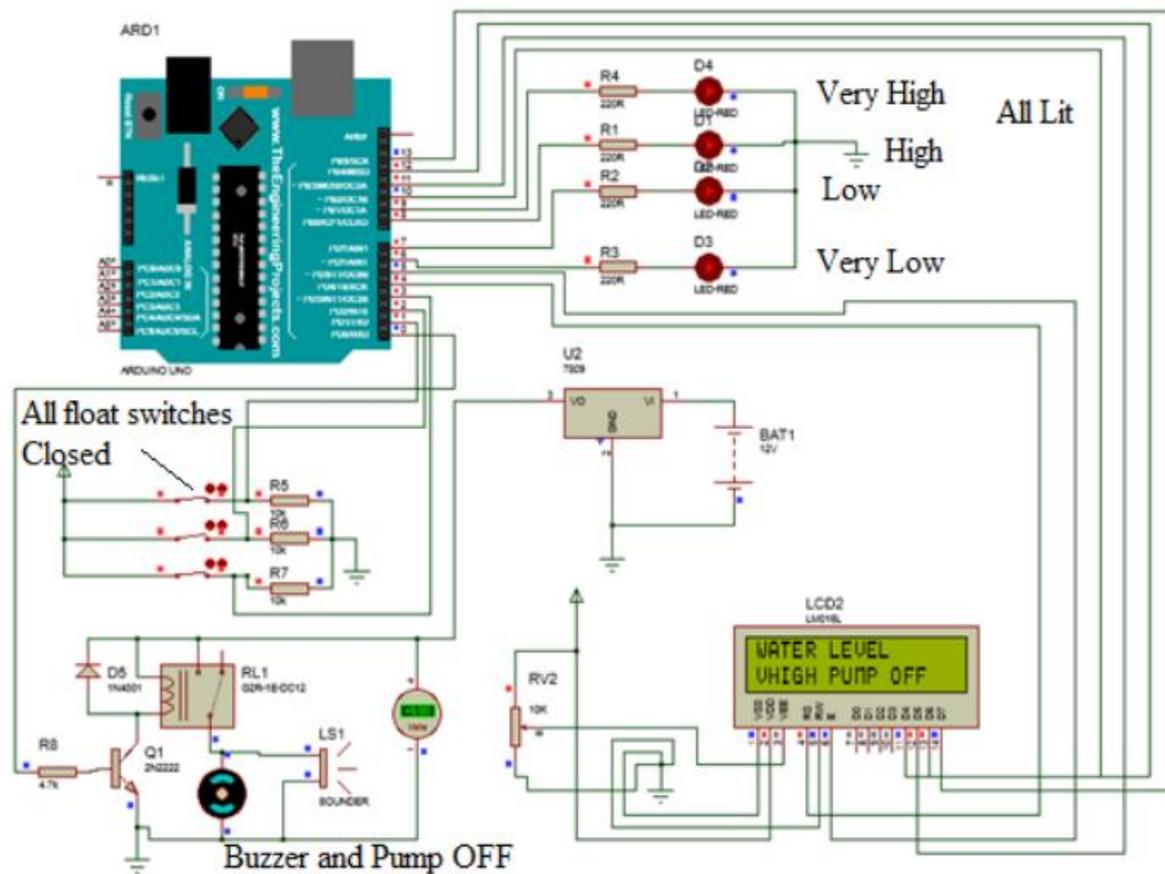
Fig. 6 Simulation in proteus environment.
