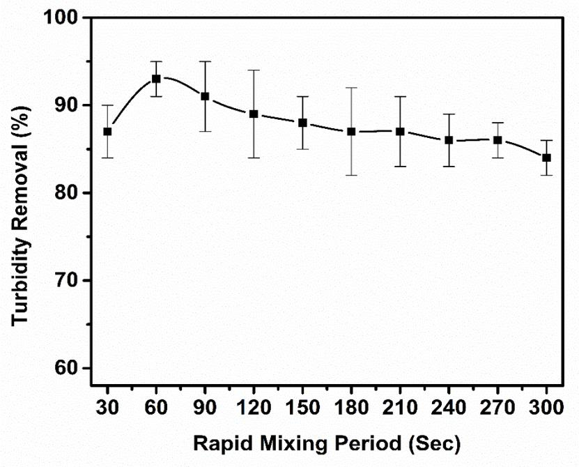
Fig. 5. Effect of Rapid mixing period on turbidity removal.
