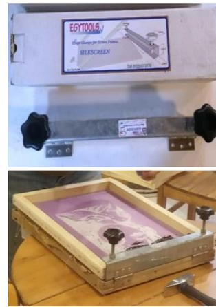
Figure 27, Using the hinge clamps to produce colored prints and controlling the color effects, on A4 paper. | Figure 28, Hinge clamps, designed by the researcher.
