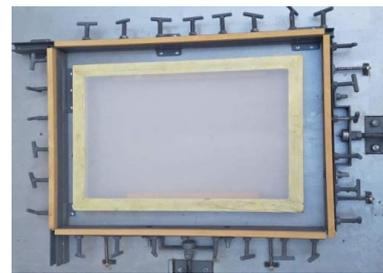
*Figure 16, A Stable Oblique Tensile Angle Stretching Machine. Designed and made by the researcher.*
