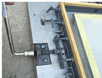
*Figure 15, Stretching process in being implemented in an oblique angel by using wooden pieces and dragging machine, composed of rolling bearings and a Spanish steel axis.*
