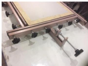
*Figure 17, Stretching process in being implemented in an oblique angel by using wooden pieces and dragging machine, composed of rolling bearings and a Spanish steel axis.*
