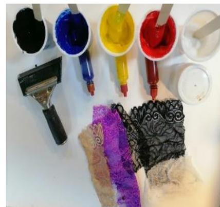
*Figure 30, Transparent printing pastes by adding a thickener to distilled water, water pigment and some effects.*
