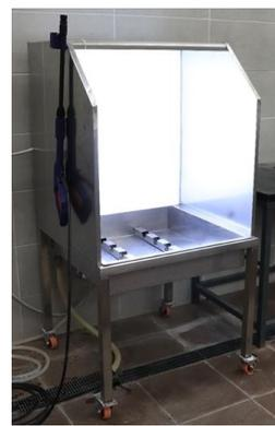
Figure 26, 304 mm Stainless Steel Backlight Washout Booth, invented by the researcher.
