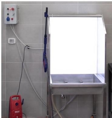
Figure 25, IP control panel separated from the machine and a 130 BAR water pump.
