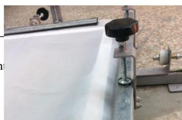
*Figure 19, Stretching process in being implemented in a horizontal pose, and could be fixed and used on any surface.*
