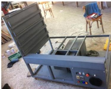
*Figure 11, Grand Drying Cabinets, it was designed to be dismantled and reassemble easily for transportation, because of its big size. 100x70cm*
