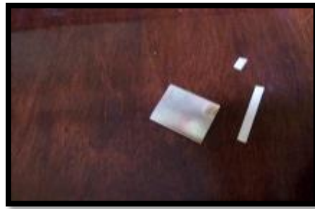
Figure 8 Detachment of inlaid units
