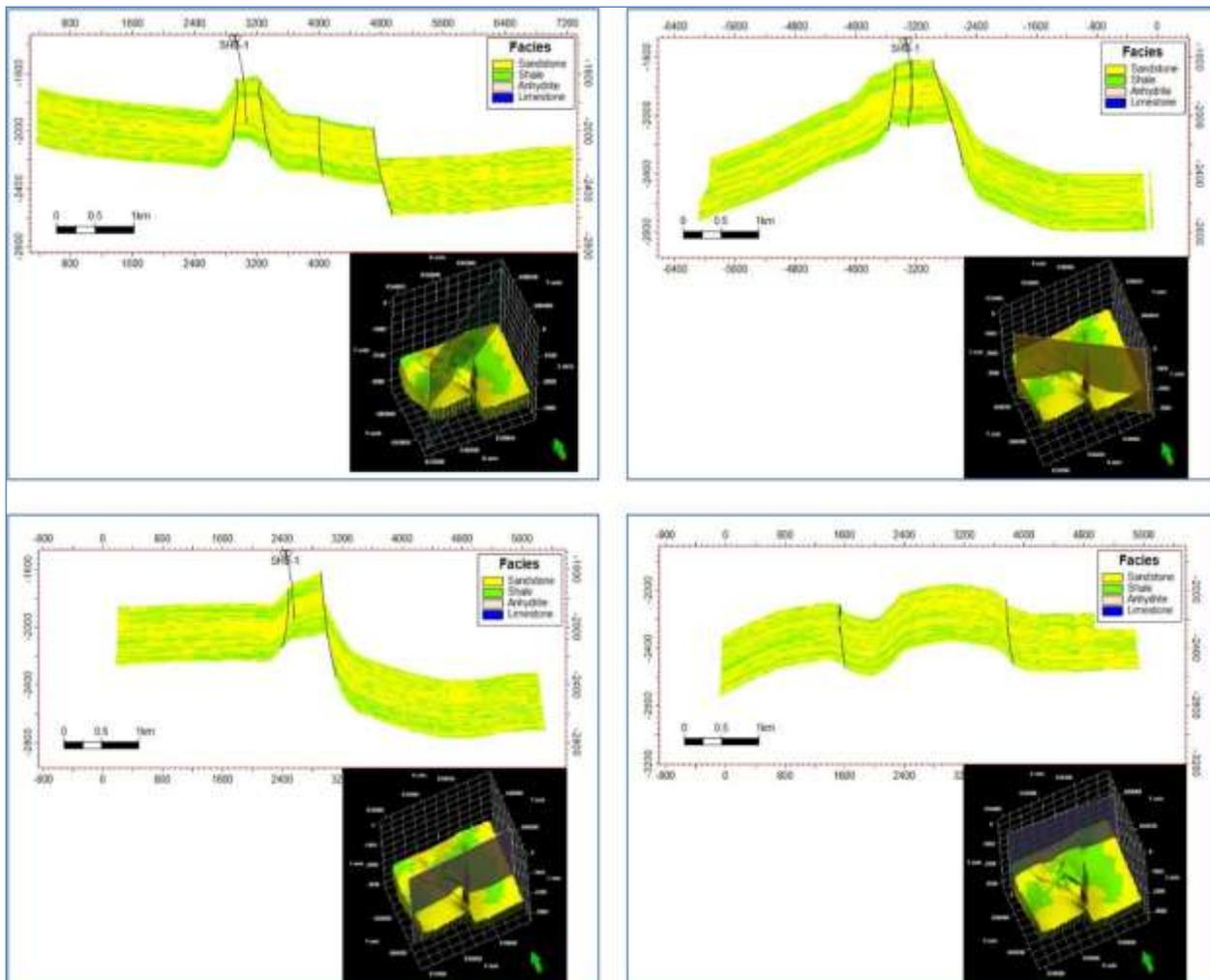
**Fig. (10):** Four Cross Sections Along the Facies Model for the Lower Rudeis Sandstone
