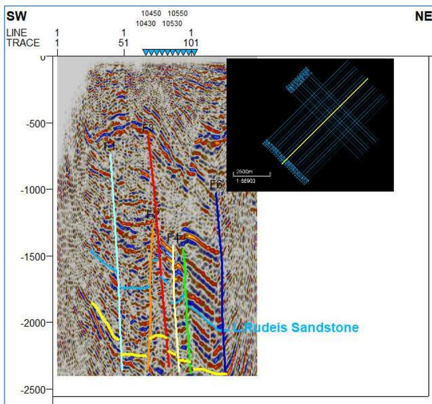
**Fig. (6):** A Seismic Section Shows the Picked Lower Rudeis Sandstone Horizon
