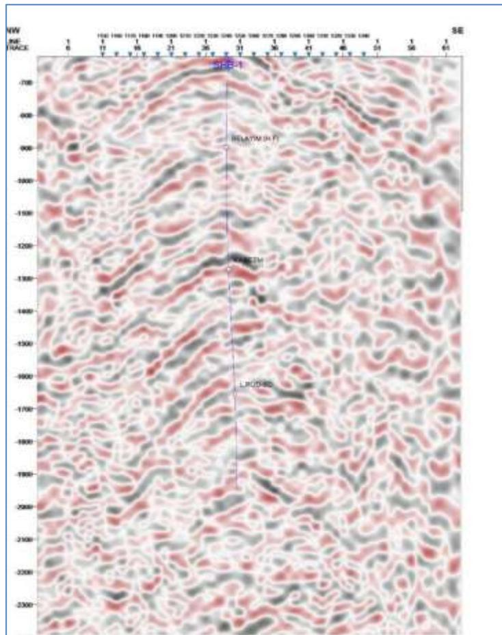
**Fig. (5):** A Seismic Section Tied to a Well
