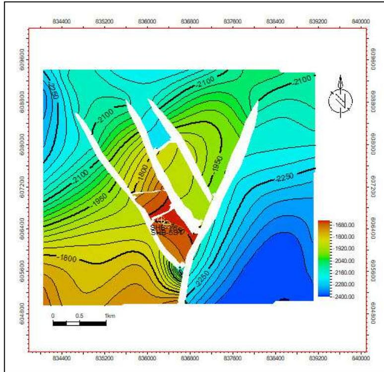
**Fig. (7):** Depth-Structure Contour Map for the Lower Rudeis Sandstone
