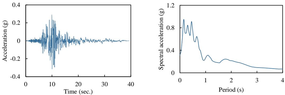
Fig. 11. Acceleration history and response spectrum of the Imperial Valley 1979 earthquake.
