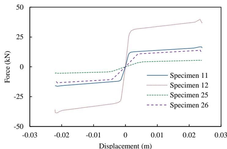
Fig. 3. Skeleton curves of shear force and shear displacement for the vertical shear links
