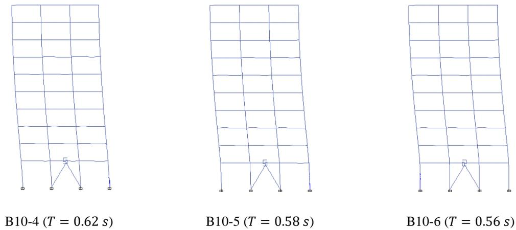
Fig. 6. First mode shape of the ten-story configurations.
