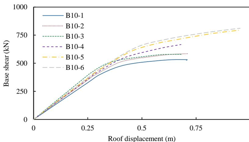
Fig. 9. Pushover curves for the ten-story configurations.
