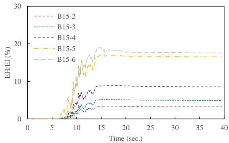
Fig. 20. Ratio of dissipated energy to earthquake input energy for the fifteen-story building configurations.
