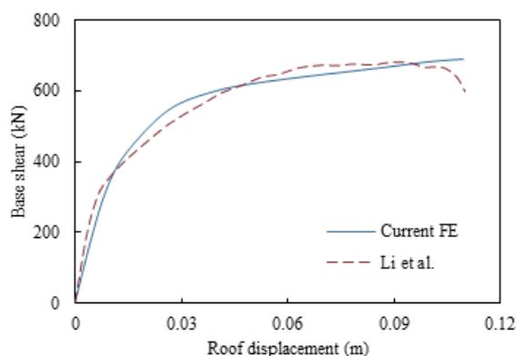
Fig. 4. Comparison between the experimental pushover curve reported by (Li et al., 2021) and the numerical curve of the verification study.
