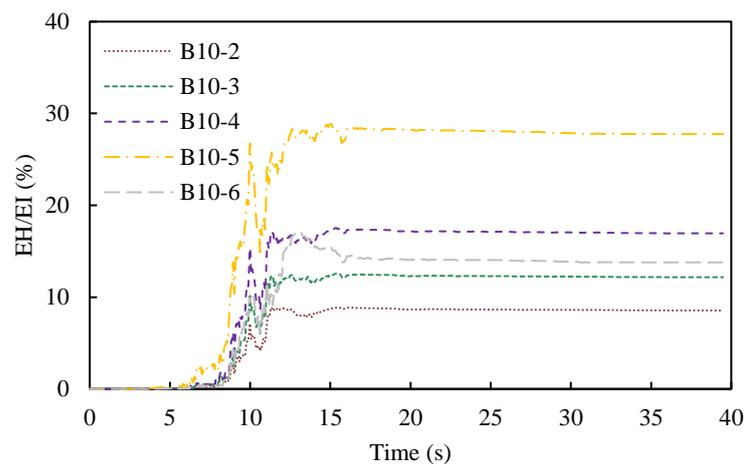
Fig. 17. Ratio of dissipated energy to earthquake input energy for the ten-story building configurations.
