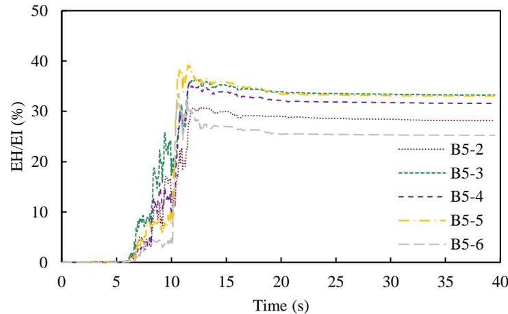
Fig. 14. Ratio of dissipated energy to earthquake input energy for the five-story building configurations.
