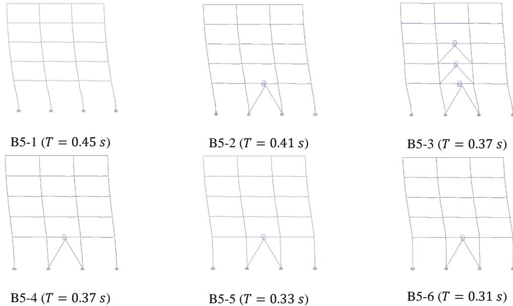
Fig. 5. First mode shape of the five-story configurations.
