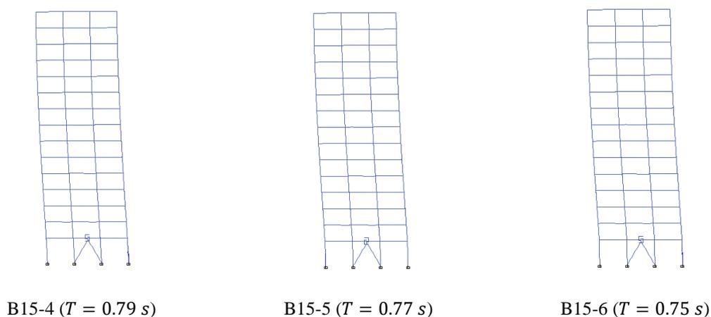
Fig. 7. First mode shape of the fifteen-story configurations.
