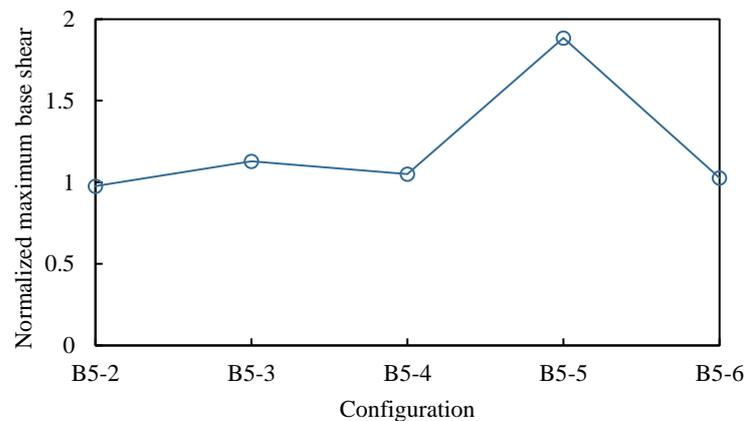
Fig. 12. Normalized maximum base shear for the five-story configurations.
