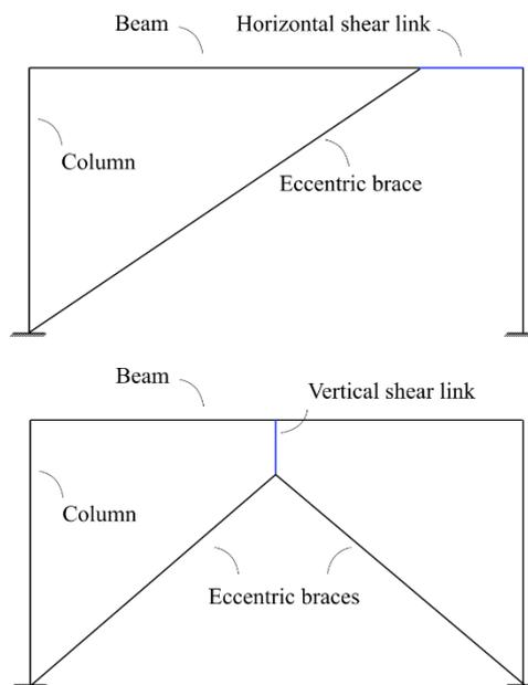
Fig. 1. Typical eccentrically braced frame.
