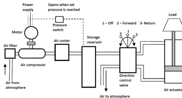
Fig.3 Components of a pneumatic system.
