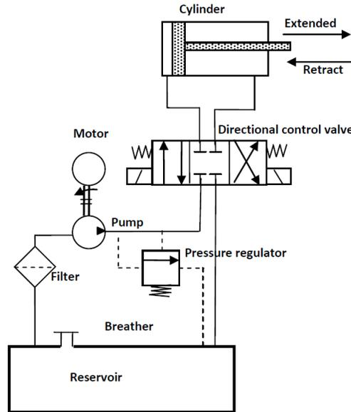
Fig.2 Components of a hydraulic system using symbols
