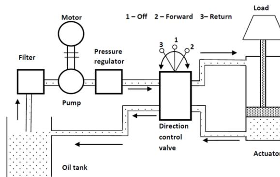
Fig.1 Components of a hydraulic system
