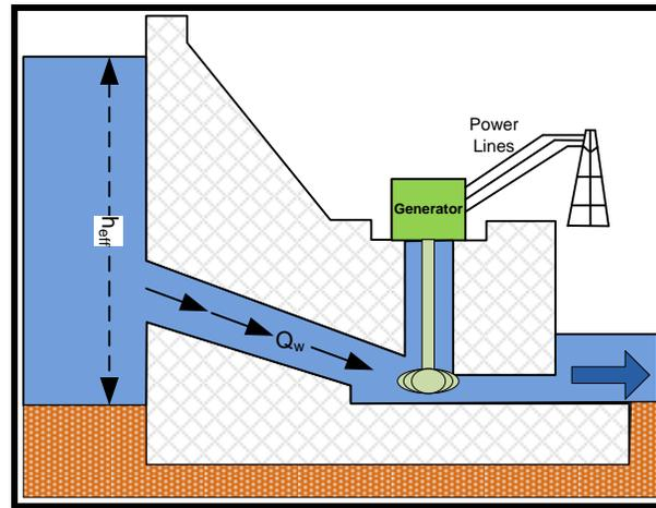
Fig. 4the hydroelectric power station
