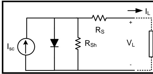
Fig. 2 Equivalent circuit for solar PV
