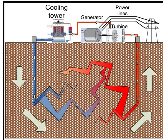
Fig. 5 the geothermal planet
