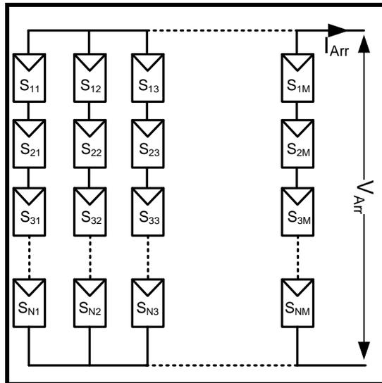
Fig. 3: solar cell array N series cell and M parallel string
