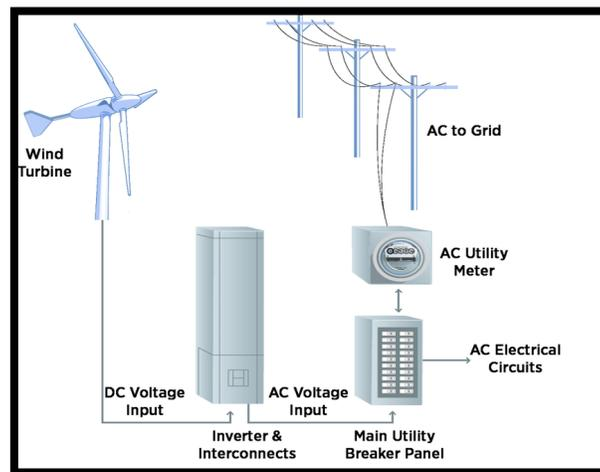
Fig .1 : wind turbine connected to the grid
