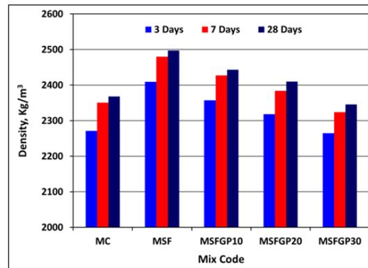
Figure 5: Densities of concrete mixes at ages of 3, 7 and 28 days
