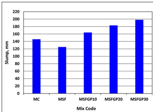
Figure 4: Slumps of concrete mixes
