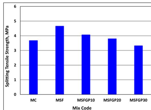
Figure 7: Splitting tensile strengths of concrete mixes at age of 28 days
