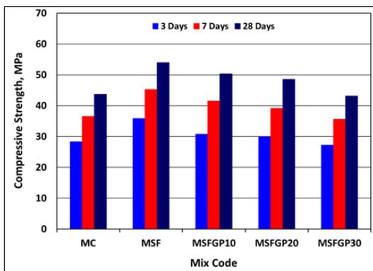
Figure 6: Compressive strengths of concrete mixes at ages of 3, 7 and 28 days
