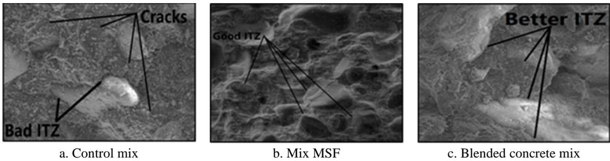
Figure 9: ITZ of concrete mixes
