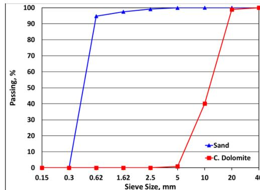
Figure 3: Sieve analysis test of sand and crushed dolomite
