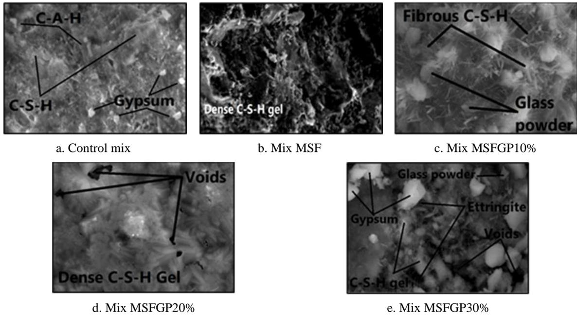
Figure 8: SEM of concrete mixes
