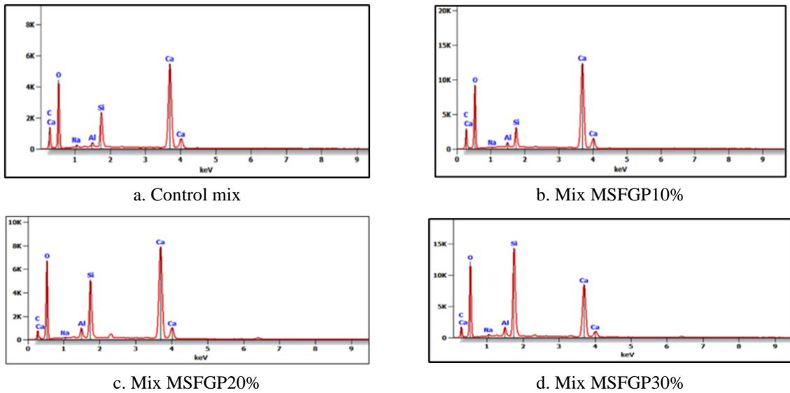
Figure 10: EDX analysis of concrete mixes
