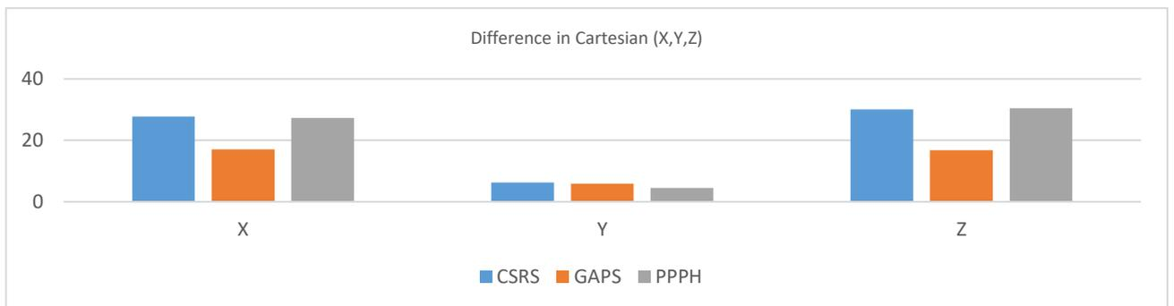
Fig 4 Difference in Cartesian coordinates between reference stations, online solutions and PPPH
