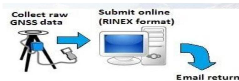
Fig 1 Online Based GNSS Processing Method
