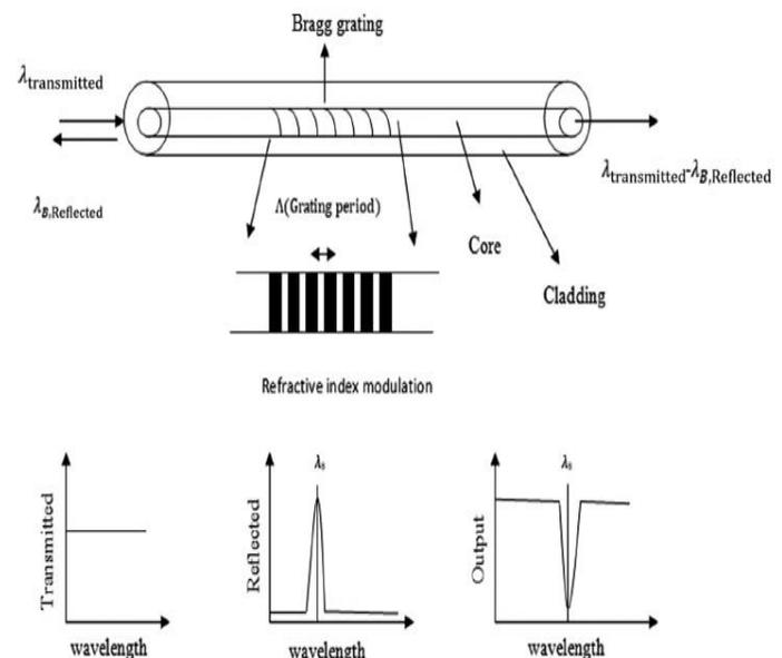
Fig. 1: Spectra of the transmitted, reflected, and output waves as well as the fiber Bragg grating structure.
