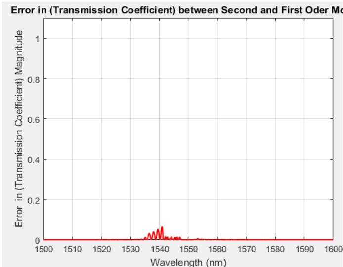
Fig 8: Error in transmission coefficient between second and first order model.
