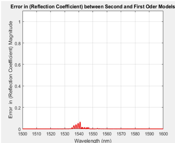
Fig 9: Error in reflection coefficient between second and first order model.
