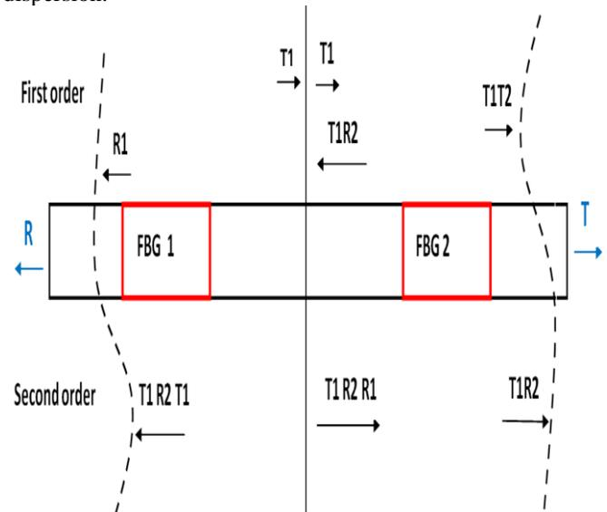
Fig 3: Two cascaded uniform FBGs.
