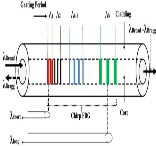
Fig. 2: A chirped FBG's configuration as a dispersion compensator.
